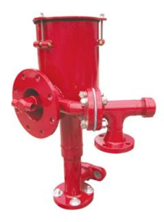
The Dual-Agent Foam Chamber from WILLIAMS FIRE & HAZARD CONTROL is a direct response to a challenge discovered in the field mitigating fires in internal floating roof tanks. It is one tool that addresses both threats occurring during an internal floating roof tank fire — the surface fire (fuel-in-depth), and the potential vapor air explosion due to residual flammable vapor above the pan.
